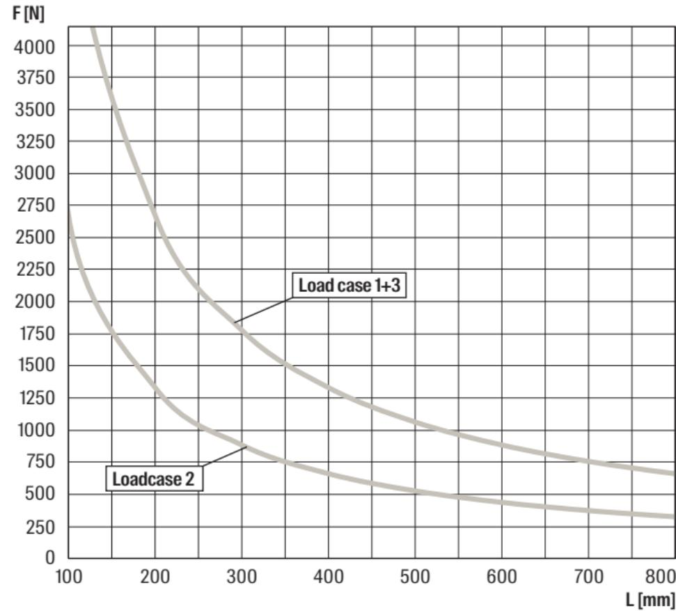
For the load curves, the permissible steel strain  $\delta_{\text{adm.}} = 160 \text{ N/mm}$  and the maximum deflection under load  $L/150$  are not exceeded. Load values of the cantilever arms under consideration of the load capacity of the base plate. Fixings and screw fastenings must be calculated accordingly. The load curves are valid for all material thicknesses of the FCA brackets.
